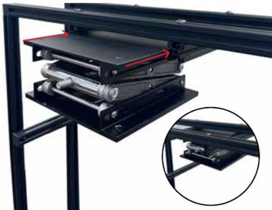
13. Insert the 150 x 150 PTZ scissor lift (Item G) in between the extrusions (1 & 2) as shown above.
